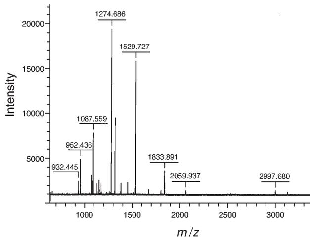
Figure 2. MALDI-TOF spectrum of a mixture of peptides obtained from tryptic digestion of hemoglobin (human).
